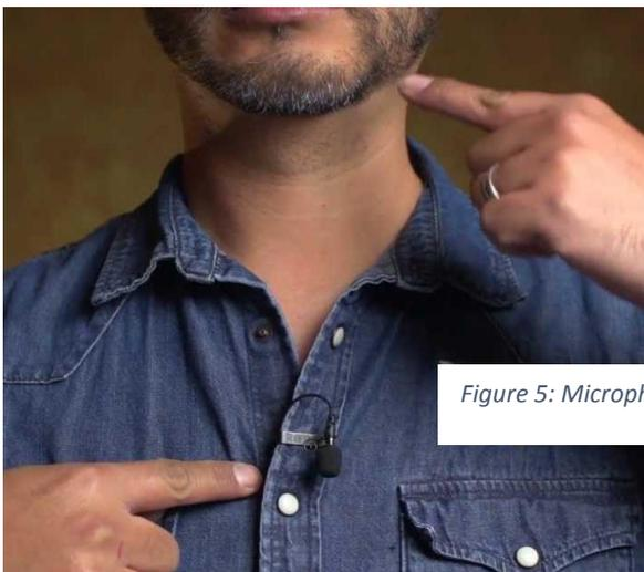
Figure 5: Microphone position
